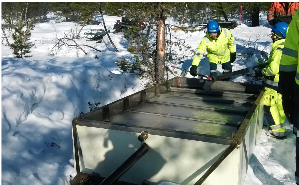
Mobile basin for sedimentation of drill cuttings.
