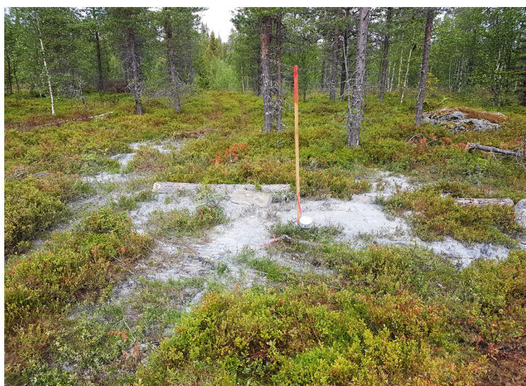
Example of drill cuttings at a site where drilling has been completed.
